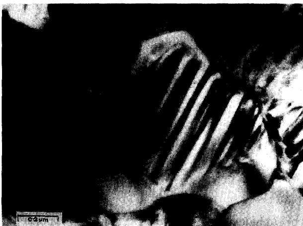
Fig. 7. TEM micrographs of sample of Type B showing (a) the grain size and duplex structure, and (b) detail of the core-shell structure (type I).
