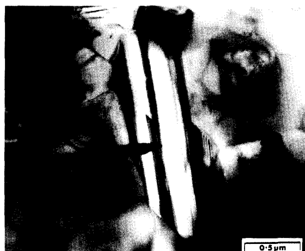
Fig. 3. TEM micrograph of second phase (arrowed) in sample of type A.
